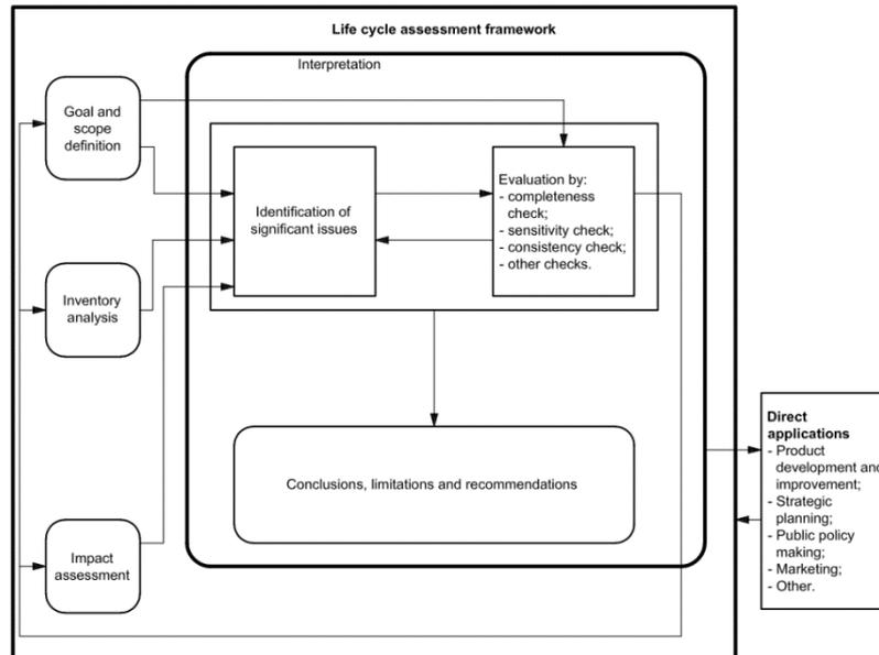
Figure 20: Relationships between elements within the interpretation phase with the other phases of LCA
