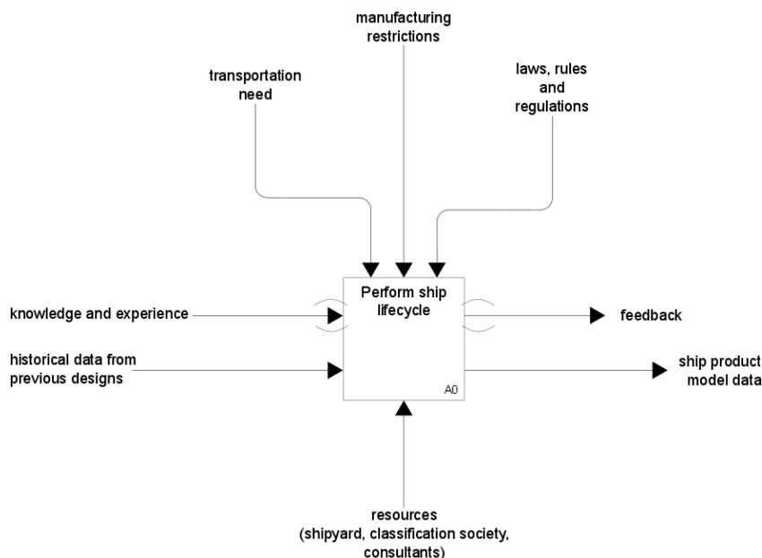
**Figure 5: Ship Life Cycle Activity Model [ISO 10303]**
