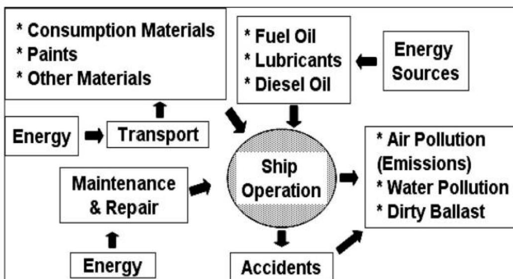
Figure 13: Ship operation flows and boundary
