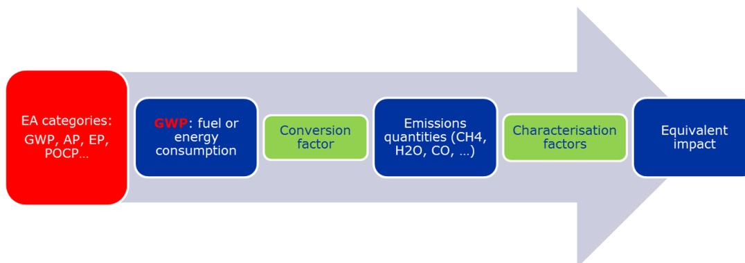
**Figure 15:Flowchart of characterisation method principle**
