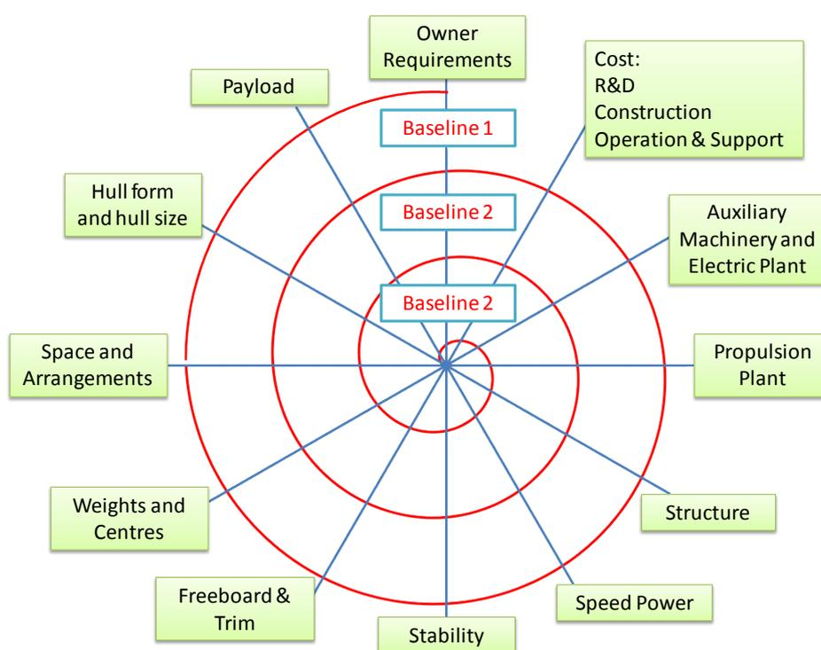
**Figure 1: Design spiral based on (Gale 2003)**
