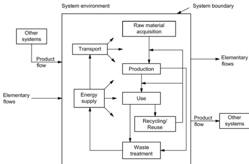
Figure 21: Example of a product system for LCA
