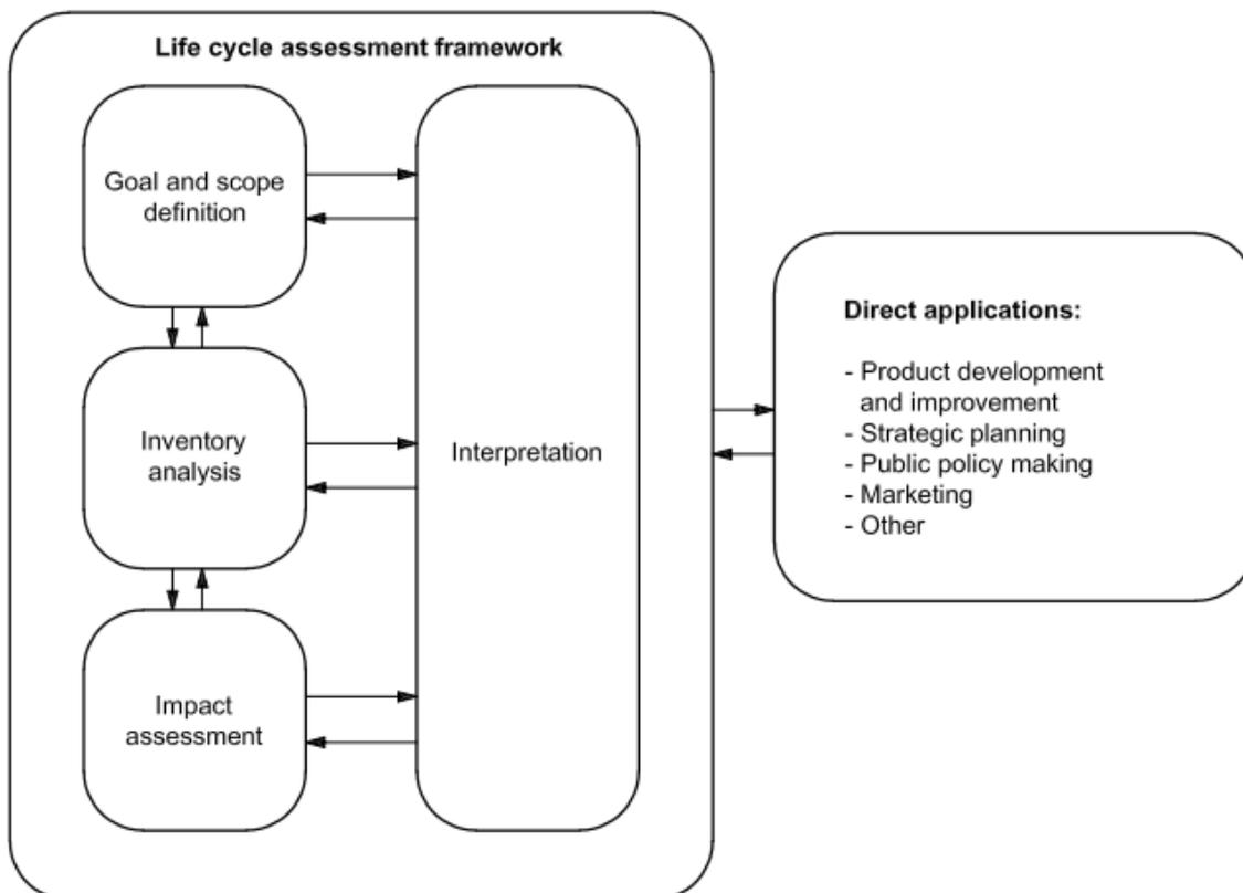
Figure 17: Stages of an LCA
