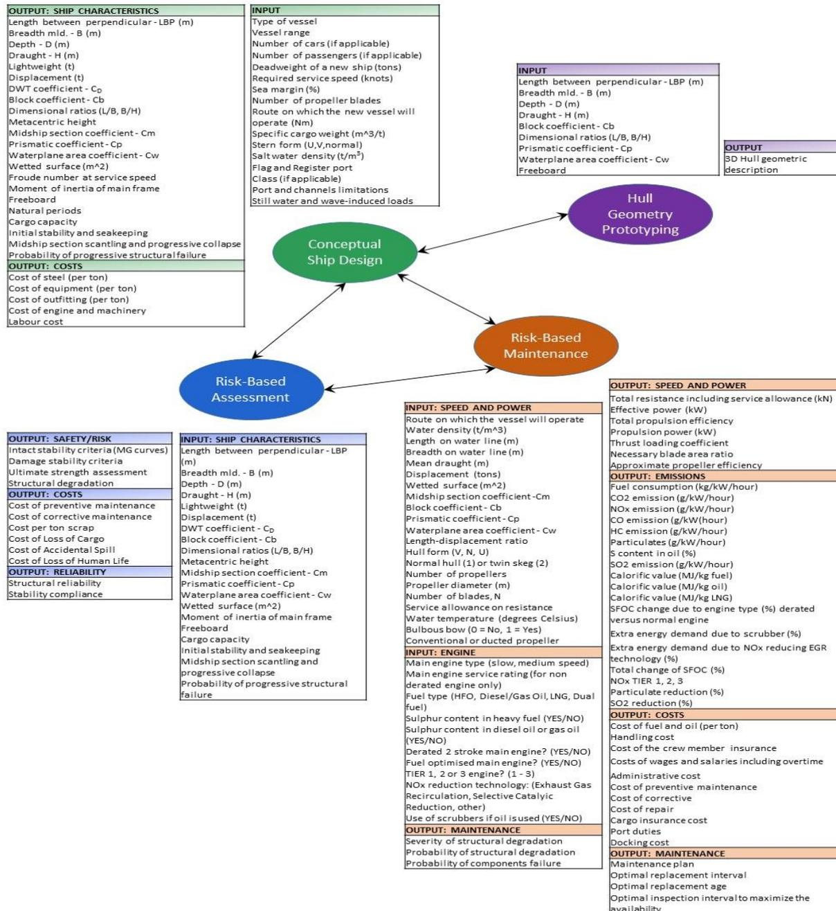
Figure 29: Indicative list of Input-output parameters
