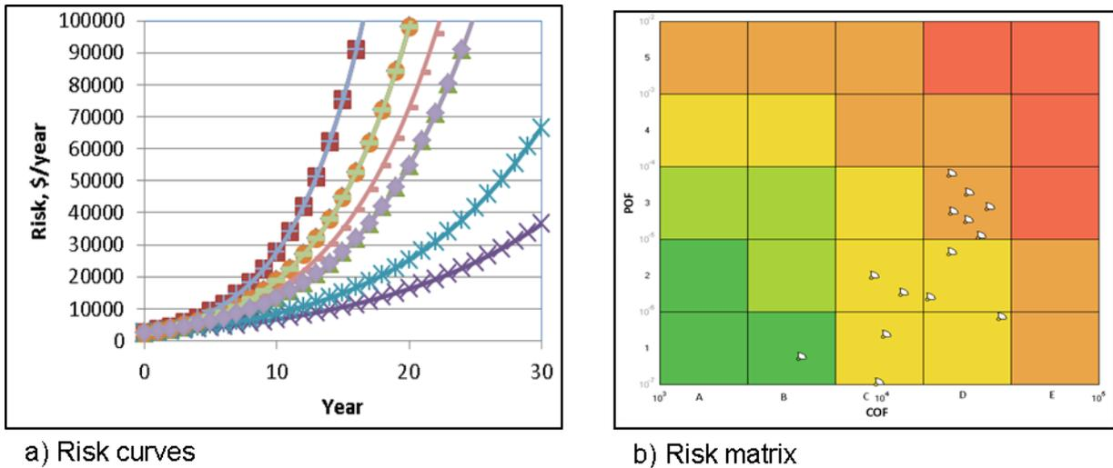
Figure 16: The example of a) risk curve and b) risk matrix for demonstration of RA assessment in RiskWISE®.
