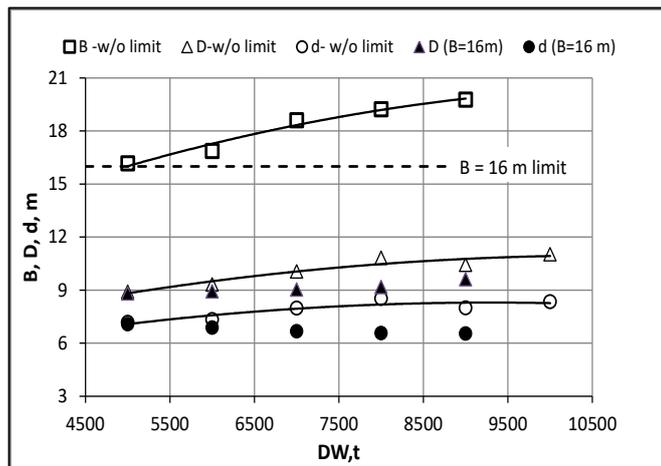
Figure 3 Main dimensions B, D, d as a function, of DW
