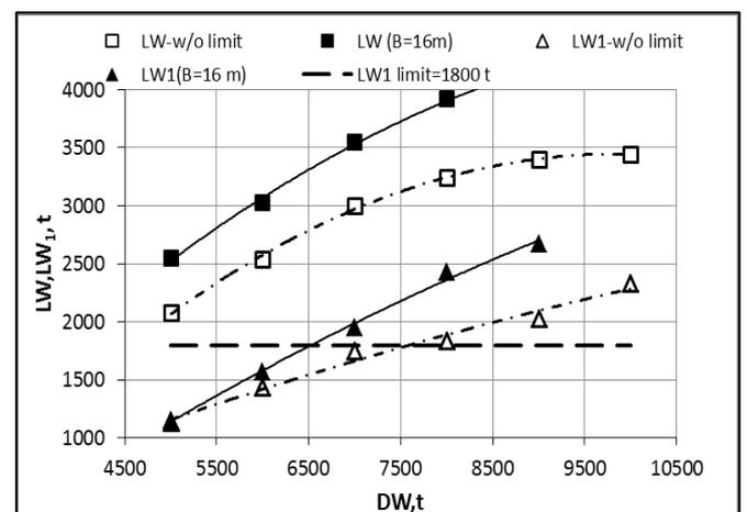
Figure 5 Light weight  $LW$  and  $LW_1$  as a function of DW
