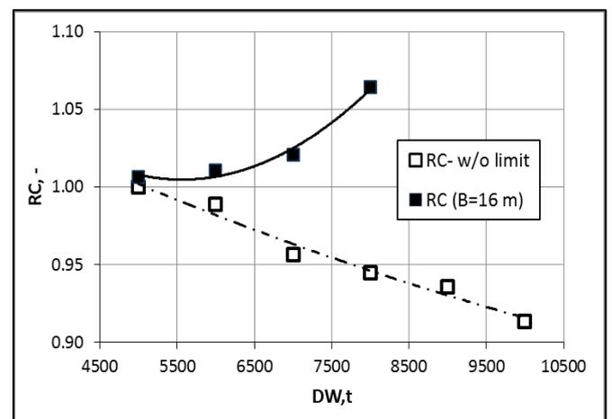
Figure 6 Relative CAPEX (RC) as a function of DW, t and influence of B limit.
