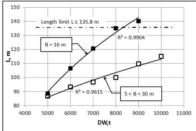
Figure 2 Main dimensions as a function of DW ( $L < 135.8$  m)
