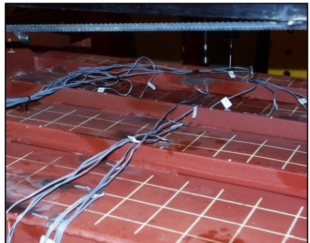
Figure 8 - Collapse's stage: magnification of out of plane deformations on the top panel under compression
