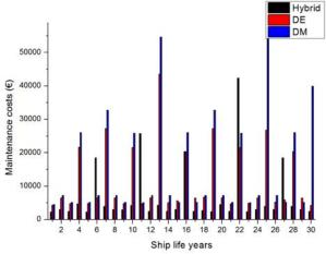
Figure 7 Engine maintenance costs over ship life years
