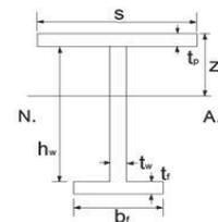
Figure 2 T-type stiffened plate cross-section
