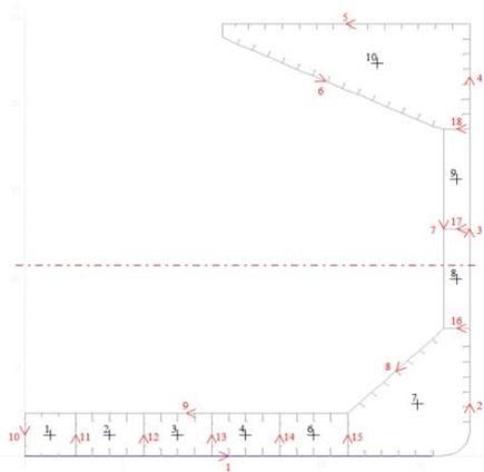
Figure 1 Half cross section of ship hull
