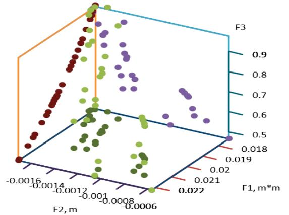
Figure 4 Pareto frontier solution: F1-net section area vs F3-fatigue damage vs F2-deflection.
