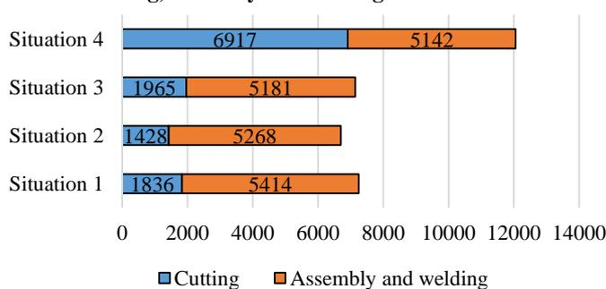
Figure 12 - Cutting costs, in [€], of the implementation of different cutting technologies in block B.
