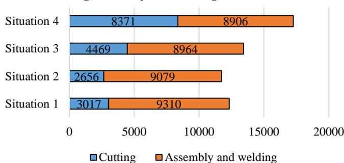
Figure 11 - Cutting costs, in [€], of the implementation of different cutting technologies in block A.
