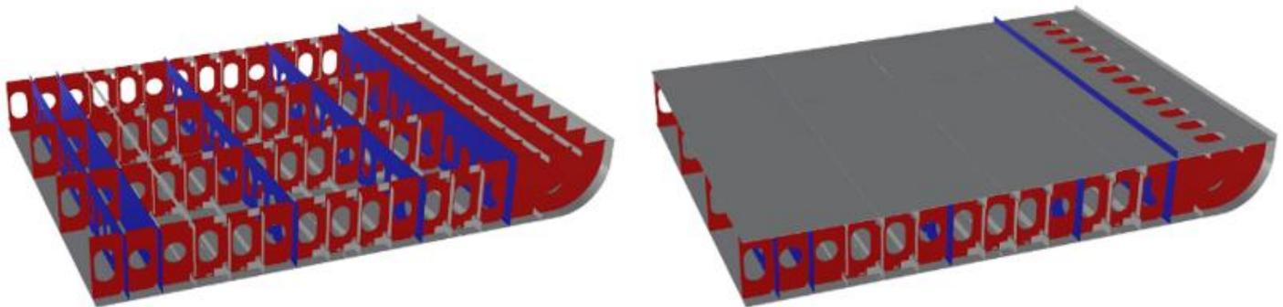
Figure 10 – Block B – double bottom block
