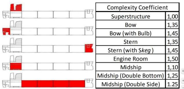
Figure 2 – Block complexity coefficient. (Leal & Gordo, 2017)
