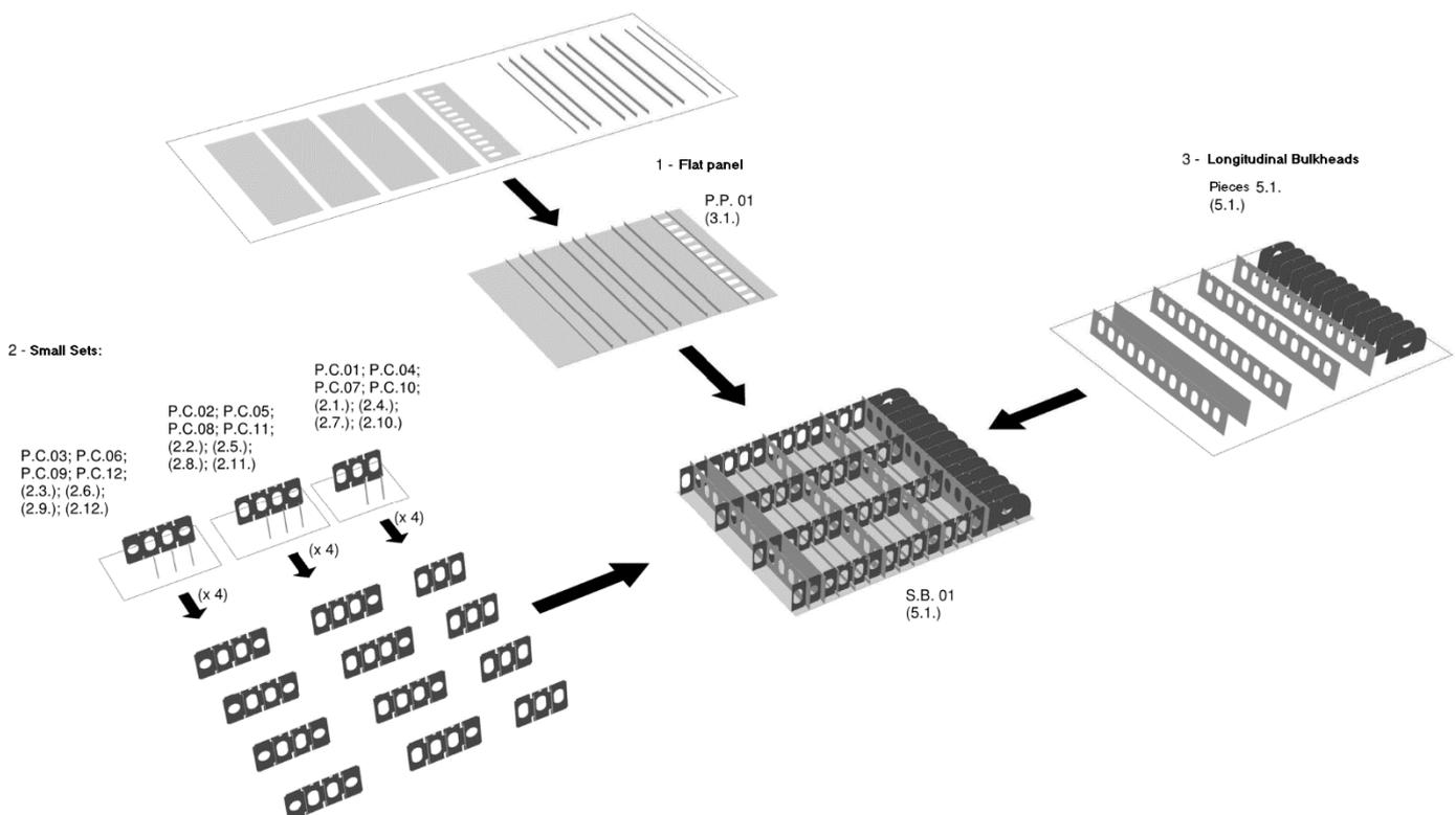
Figure 6 – Block construction sequence
