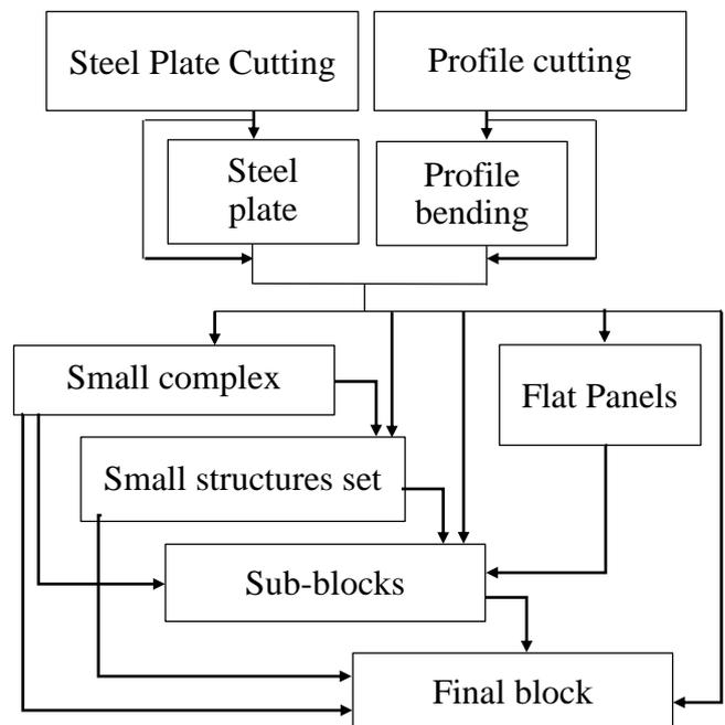
Figure 1 Block production sequence main stages scheme
