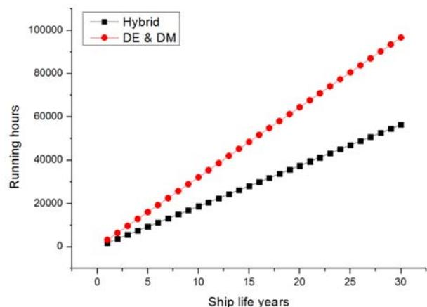
Figure 6 Running hours or each engine vs operation years
