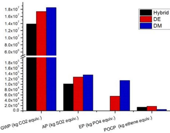
Figure 10 Results of LCA
