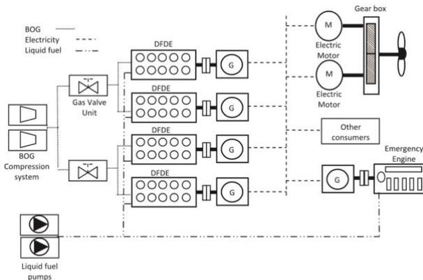
Fig. 14. Configuration of diesel-electric propulsion using DF engines (4S).
