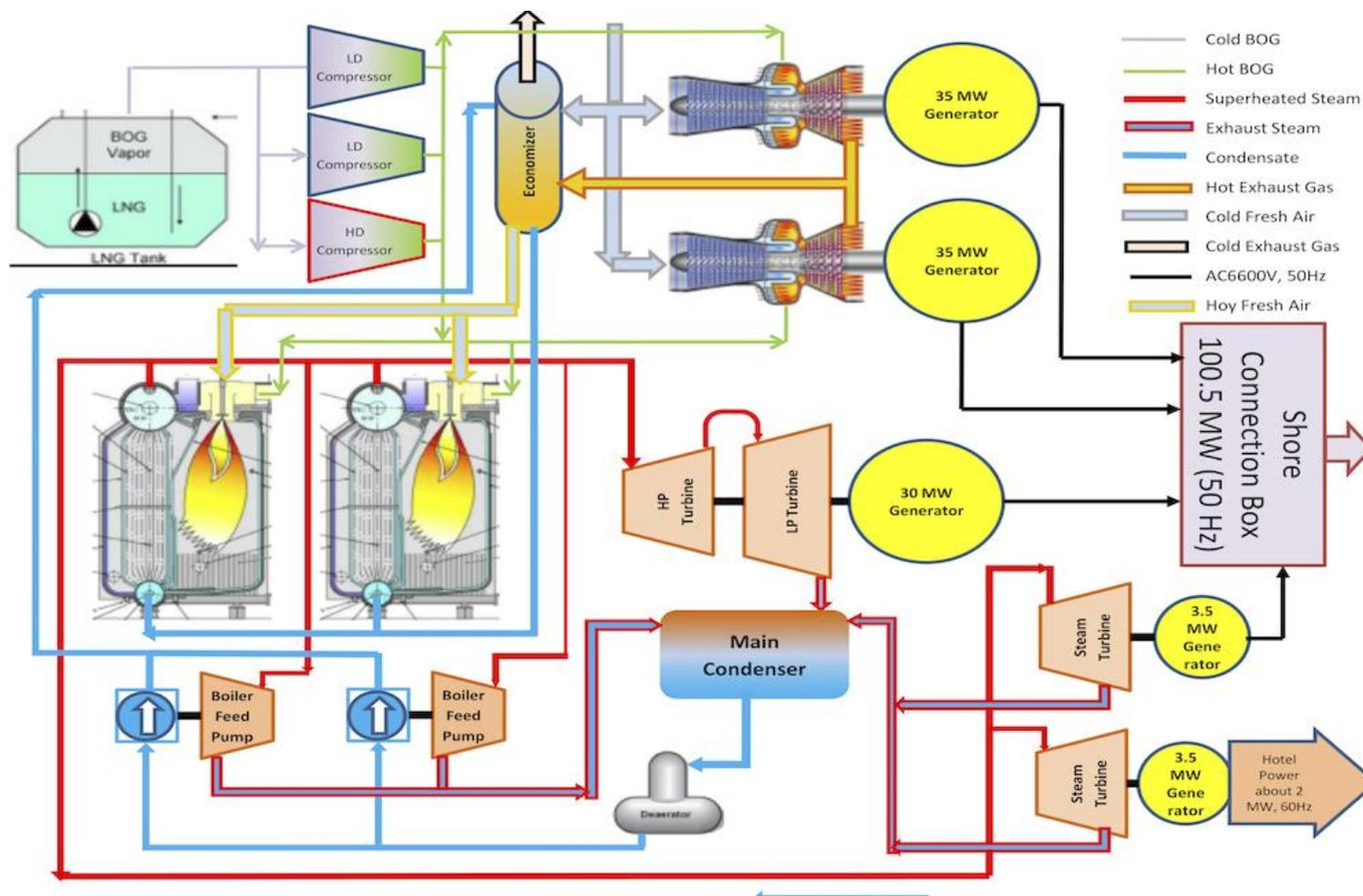
Figure 7. Steam turbine FPGP arrangement
