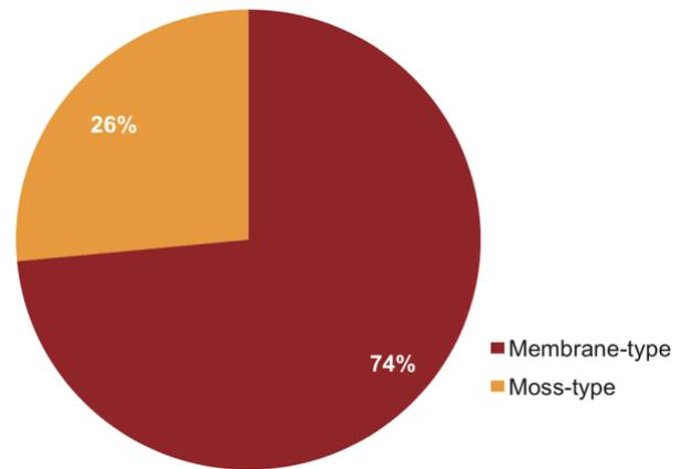
Figure 5. Existing fleet by type of containment system by the end of 2017 [2]
