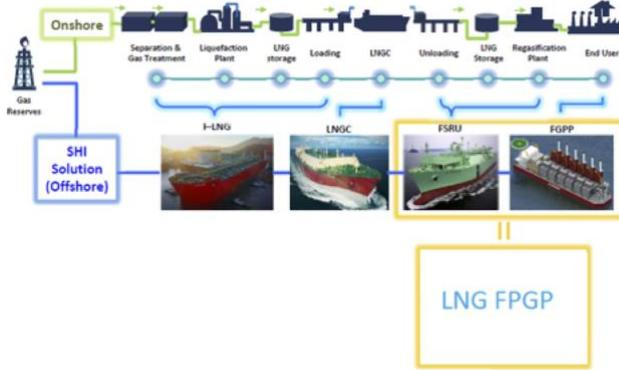
Figure 6. The FPGP in the natural gas supply chain
