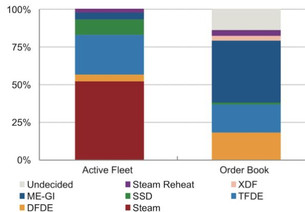
Figure 1. LNGC fleet by type of propulsion system by the end of 2016 ([2])
