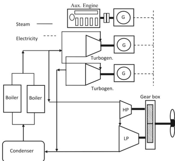
Fig. 3. Configuration of a basic propulsion system through an ST.
