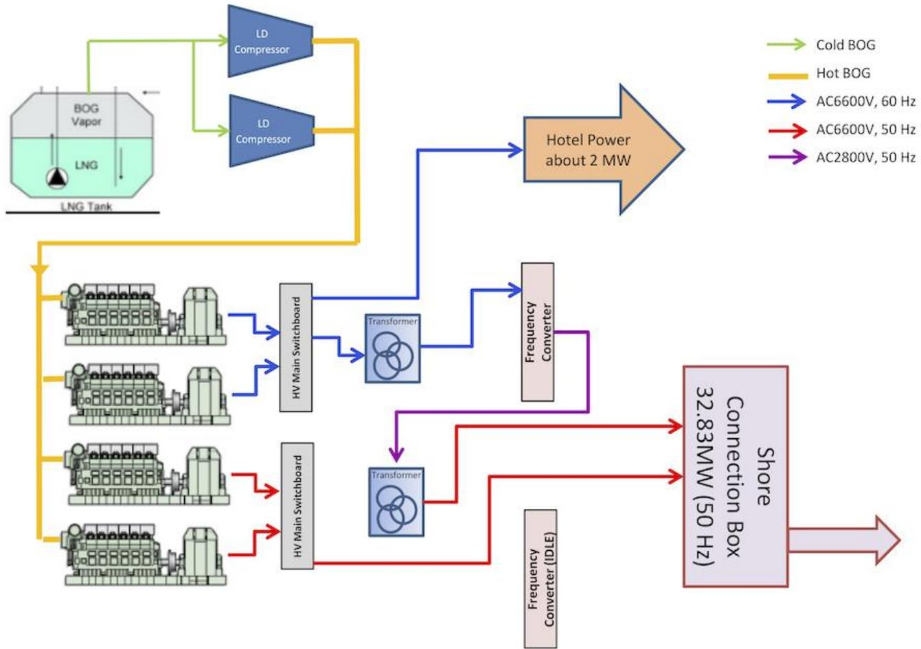
Figure 8. D/TFDE FPGP arrangement
