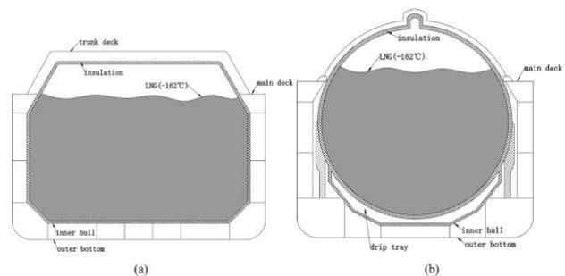
Figure 3. Typical conceptual drawing of membrane (a) and MOSS (b) containment systems [4]
